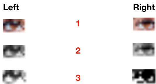
Figure 3. Eye data is scaled down (1), then converted to greyscale (2), and then the greyscale image is normalised (3).
